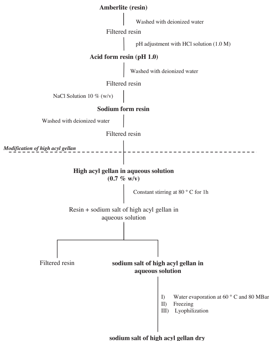
Fig. 2. Preparation of NaHAG from LT-100.
